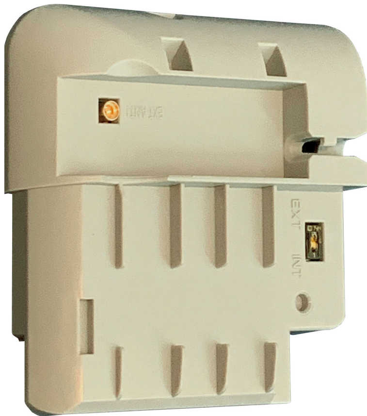
Figure D.1: A Cellular Module
